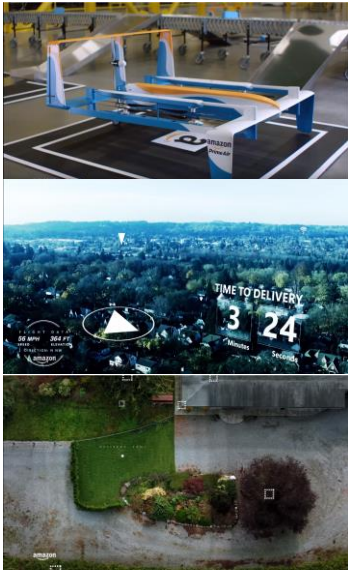
Figure 3: Screenshots from the Amazon Prime Air concept video, showing the actual drone (top). While the drone is in horizontal “plane” mode (middle), the video shows the drone’s point-of-view by facing the camera horizontally, not identifying features of the houses it flies over. While in vertical landing mode (bottom), the camera faces vertically down, but only the package recipient’s yard is in frame. The vertical-facing camera does not show any other person’s property.
